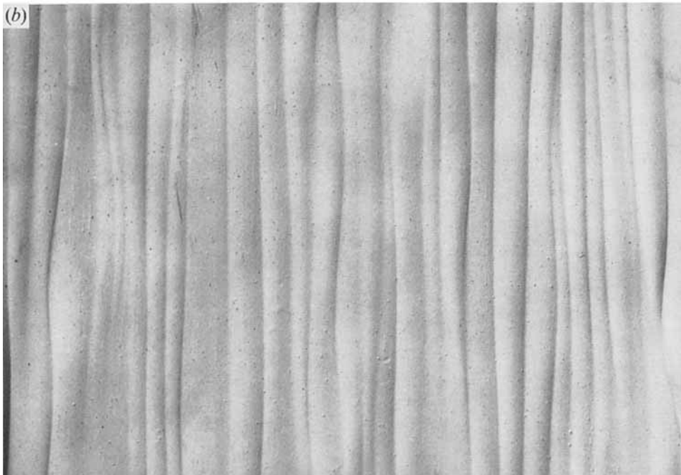
FIGURE 5. Moulds of assemblages of experimental longitudinal ridges and furrows. (a) Rectilinear furrows, (b) weakly sinuous furrows involved in higher-order instability. In each case flow is from bottom to top and width of bed shown is approximately 28 cm. See text for flow conditions.
