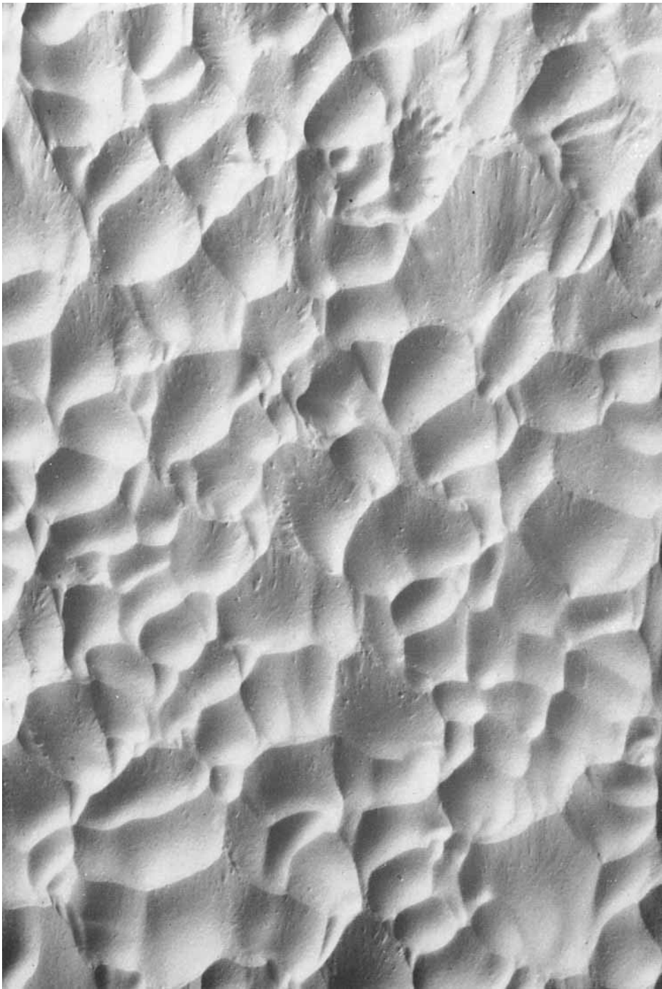
FIGURE 2. Experimental scallops developed in Plaster of Paris. Flow from bottom to top. The portion of the bed shown is approximately 17 cm wide. See text for experimental conditions. Note that the photograph shows the original bed and not a mould (cf. figures 3, 5, 7).
